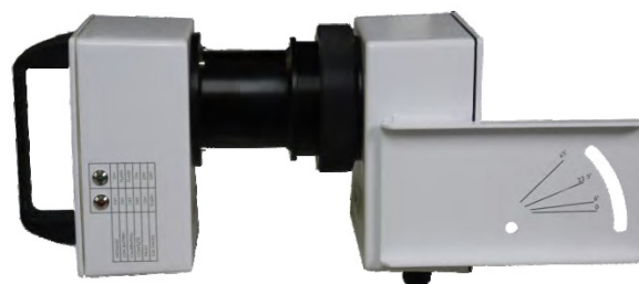
ALS-2 Calibrator connected to the ALS-2 for in situ calibration
