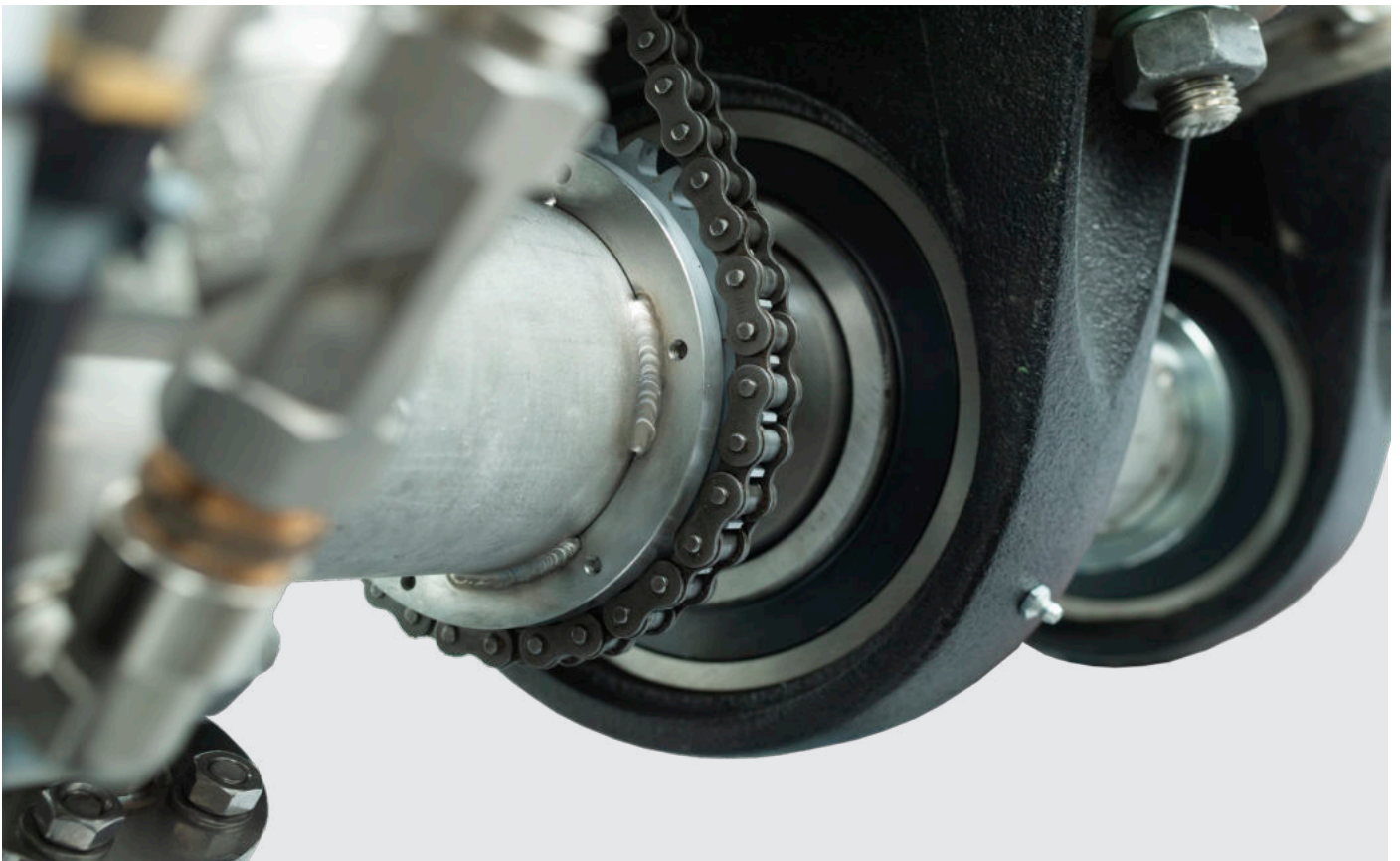
Figure: The powerful probe rotation device prevents thermal bending and sticking.
