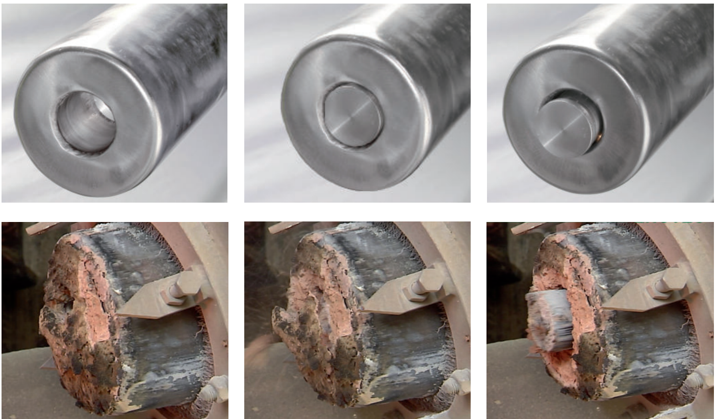
Figure: Automated plunger keeps the flue gas entrance free of blockages.
