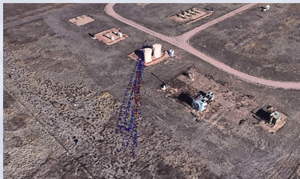
Leak plumes from a METEC storage tank are mapped in minutes using the MIRA Strato gas analyzer mounted on the underside of a DJI Matrice 600 drone. Red indicates highly correlated ethane and methane.
