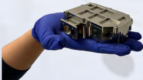
MIRA's compact optical core achieves a 13 meter path length in a 60 cc volume.
