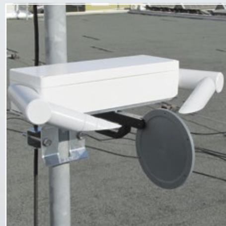
The degree of contamination of the sensor is transmitted together with the measured values and serves to alert proactive maintenance.
