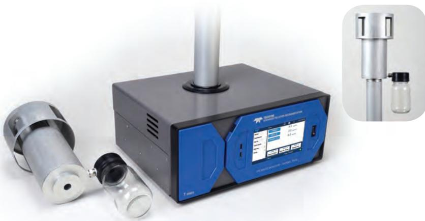
The T640 is completely self-contained and includes an internal 5-lpm vacuum pump, aerosol sample conditioner, and sample flow controller. The base model T640 is a US EPA-approved PM<sub>2.5</sub> Federal Equivalent Method.
