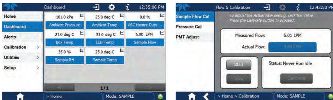
The NumaView™ software interface provides a programmable dashboard for diagnostic parameters, as well as single-point calibrations of sensors.
