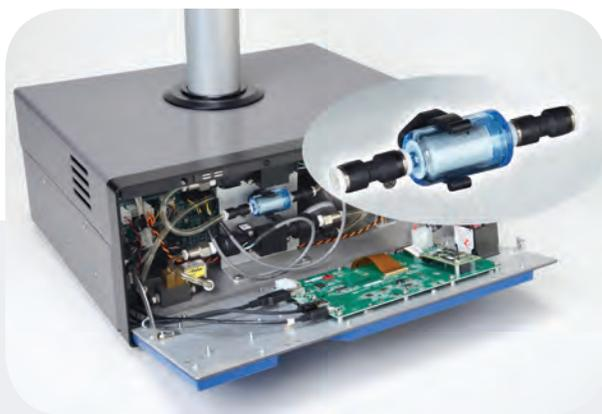
A convenient 19" rack mount chassis with front and rear panel fold down access to serviceable components. An in-line filter protects the flow sensor and pump from contamination, and is the only consumable item with a 6-month recommended replacement interval.
