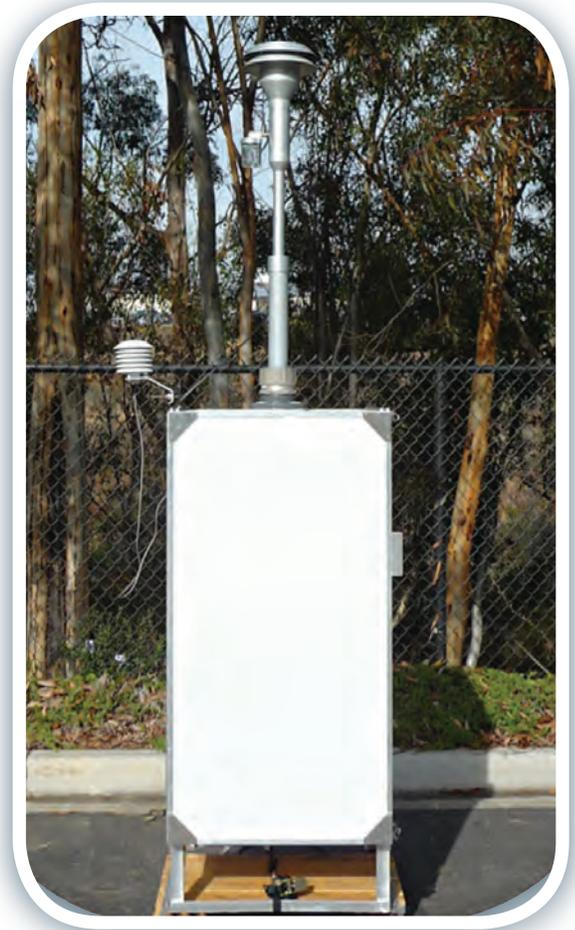
With the T640x option, the T640 can operate at 16.7-lpm and use the US EPA-approved PM<sub>10</sub> inlet. This configuration is US EPA-approved as PM<sub>10</sub>, PM<sub>2.5</sub>, and PM<sub>10-2.5</sub> Federal Equivalent Methods. (Optional environmental enclosure shown).
