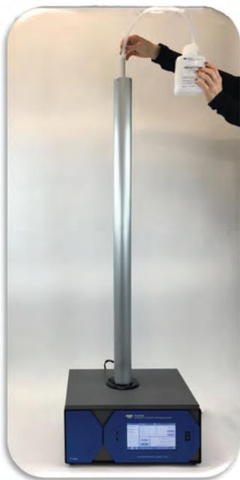
Avoid downtime from factory calibrations using our unique SpanDust™ procedure. Span verifications can be accomplished easily anytime in the field to avoid uncertainty and data loss.
