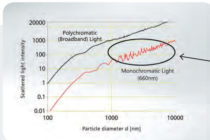
The broadband approach provides an unambiguous scattered light signal for accurate measurements over a wide particle size range.
